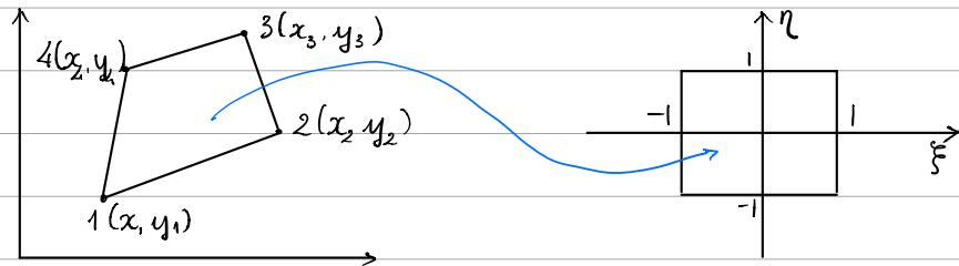
The relationship between convex quadrilateral in the physical coordinate  $Oxy$  and the standard domain  $[-1, 1] \times [-1, 1]$  in the natural coordinate  $(\xi, \eta)$  is given by :
